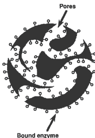
FIG. 1. Schematic illustration of immobilized enzyme molecules bound to porous supporting matrix.
